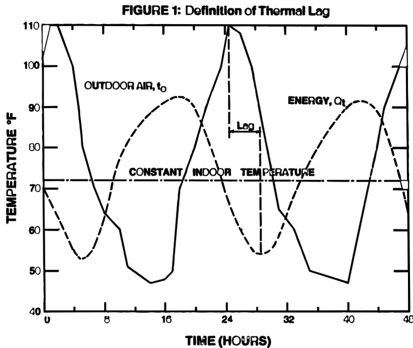
Masonry walls exhibit overall thermal performance superior to that of walls with metal framing systems with insulation of the same RSI value because their mass gives masonry walls the following advantages:
