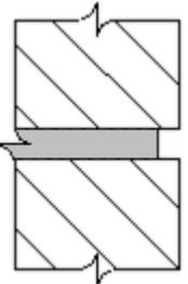
Block being laid on a horizontal “Bed Joint”
